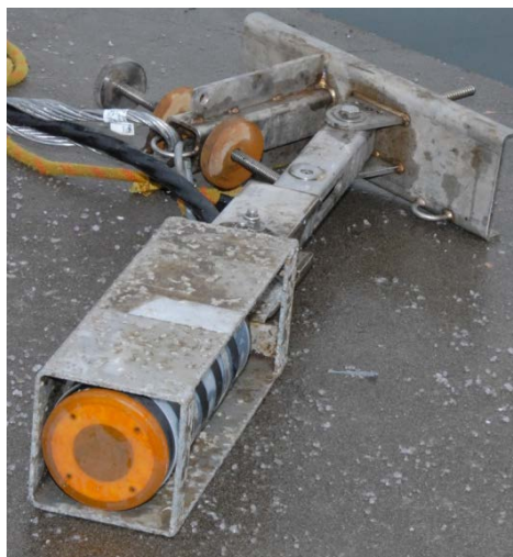
Figure 2.1. Transducer Installed in an Adjustable Mount and Prepared for Installation
